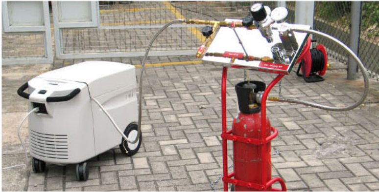
燃料電池發電機及氫氣供應設備 Fuel-cell generator and hydrogen gas supply equipment
